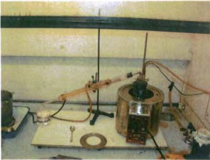
Asphalt Recovery Test
